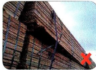
Timber load is not properly stacked and there is no lashing.
