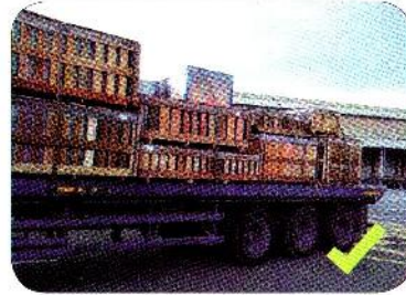
Cargoes are stacked closed to each load and secured with lashing.
