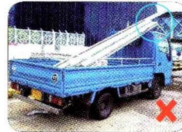
The cargo is not properly secured to the girder of the lorry.
