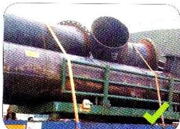
A good lashing device will secure the cargo from any movement.
