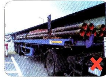
No lashing for bundled steel pipes and stanchion bar is deformed.
