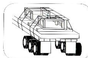
Figure 17: Use crates or steel boxes to contain and block items against the headboard of the vehicle cabin
