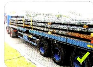
Bundles of steel rods must be properly stacked and lashed and kept within the height of the vertical girder.
