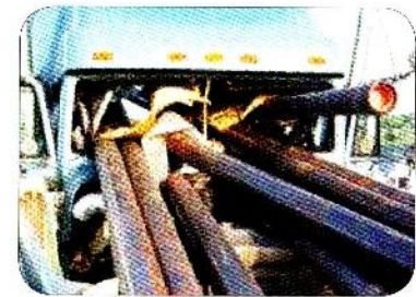
Figure 19: Pipes not properly secured and truck did not have a headboard
