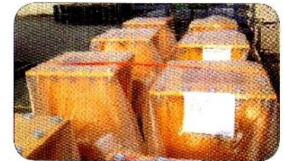
Figure 69: Tote bins on lorry, minimum front and last row must be lashed, to prevent any movement.
