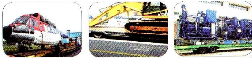
Figure 58: Usage of proper equipment and device to secure heavy and bulky cargo on low bed trailer
