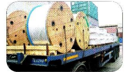
Figure 53: Cable drums must be secured by proper chocking and lashing
