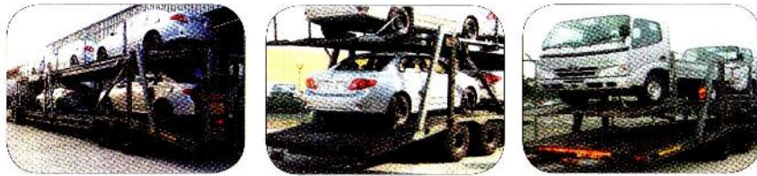
Figure 66: Ensure that proper equipment and securing devices are used for transporting cars/lorries on deck of trailers
