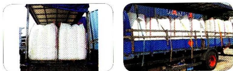
Figure 63: Jumbo bags on lorry, minimum lashing to first and last row is required
