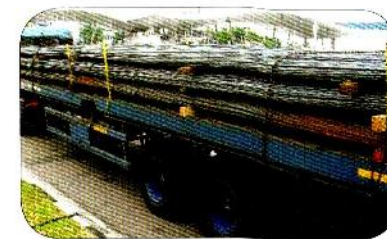
Figure 41: Sufficient stanchions/ steel bars must be fixed onto the platform and adequate lashing used on the steel pipes
