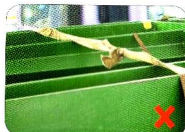
Defect lashing device should not be used as it will give way easily.
