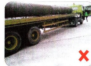
No lashing and headboard, improper and damaged stanchion bar used (cargo over stanchion bar).
