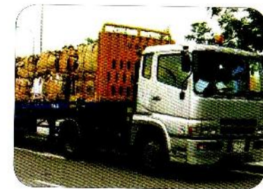
Figure 30: Trailer fixed with headboard for transporting general cargoes e.g., bundled waste
