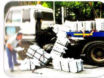
Figure 18: Tin ingots toppled from vehicle due to sudden braking and unsafe stacking
