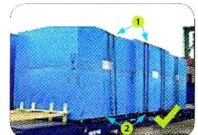
1. Padding 2. Wire ropes and tensioners are used in the unit of the load
