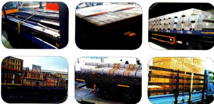
Figure 14: Placement of cargoes on lorries and trailers with tie-down to secure the cargo from movement
