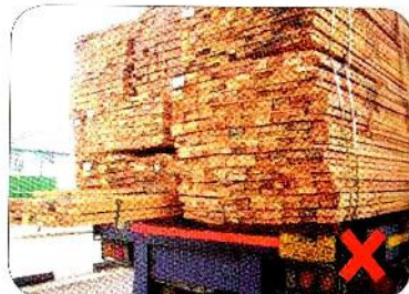
No proper indication for overlength cargo causes danger to users on the roads or at workplaces.
