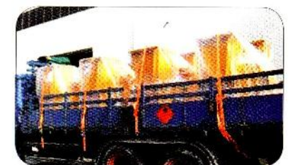
Figure 70: Metal panels on lorry, first row of cargo is placed near the headboard; the front and back rows must be lashed
