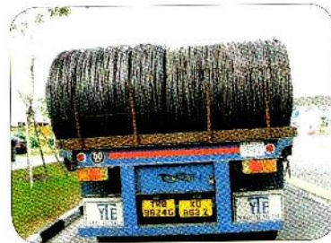
Figure 52: Vertical steel bar placed to prevent forward and rearward movement
