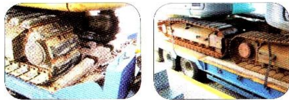
Figure 59: Proper chocking and lashing device applied to secure cargo from any movement
