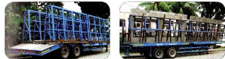
Figure 62: Trailers mounted with steel frames
