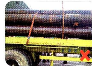
Improper stanchion used for pipe cargoes.
