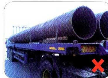
No lashing and headboard, improper stanchion bar used (cargo over stanchion bar).
